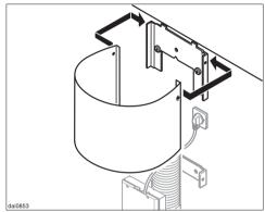
Carefully ease apart the sides of the chimney extension and hook it behind the upper retaining plate. Be careful of sharp edges.
